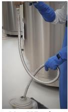
Wear PPE and use dispensing hoses made for use with cryogens.
