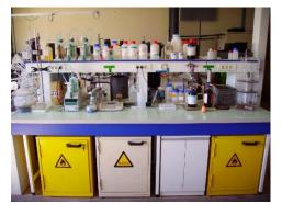
Know your cabinets! From left to right: flammable cabinet, corrosive cabinet, regular storage cabinet, flammable cabinet. None of the chemicals on the top shelf should be corrosive as the shelf is above eye level.
