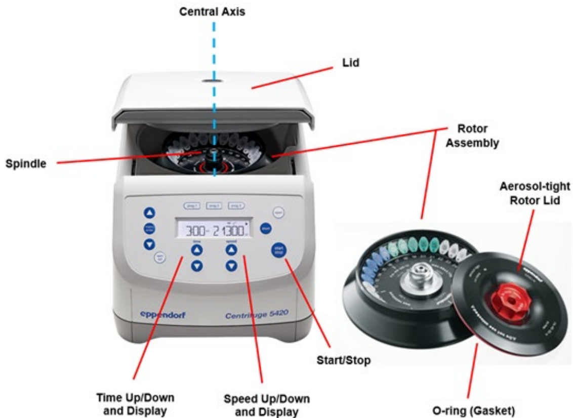
Figure 2: Labeled centrifuge with fixed angle rotor
