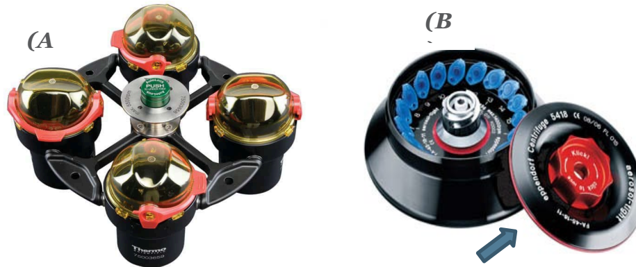
Figure 5: Example of swing bucket rotor with safety cups (A); and fixed rotor with engineered with bioseal technology (B) (O-ring indicated by blue arrow).
