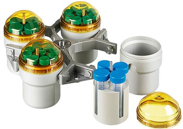
Figure 2: A) HEPA-filtered Class II biological safety cabinet for aerosol containment; B) Engineered safety cups for aerosol containment
