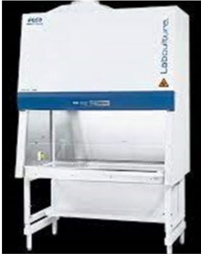
Figure 2: A) HEPA-filtered Class II biological safety cabinet for aerosol containment; B) Engineered safety cups for aerosol containment
