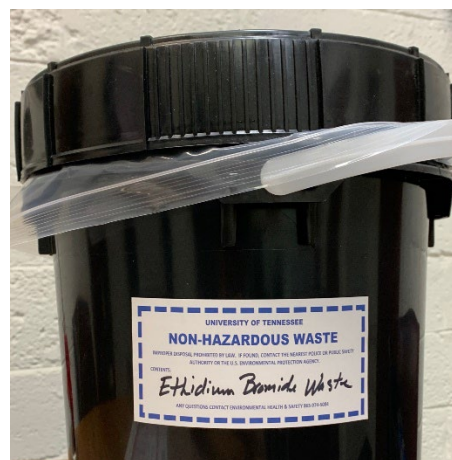
Figure 3. Example non-hazardous waste label (L) and labeled container (R) for collection of agarose gels and other solid wastes with incidental ethidium bromide contamination.
