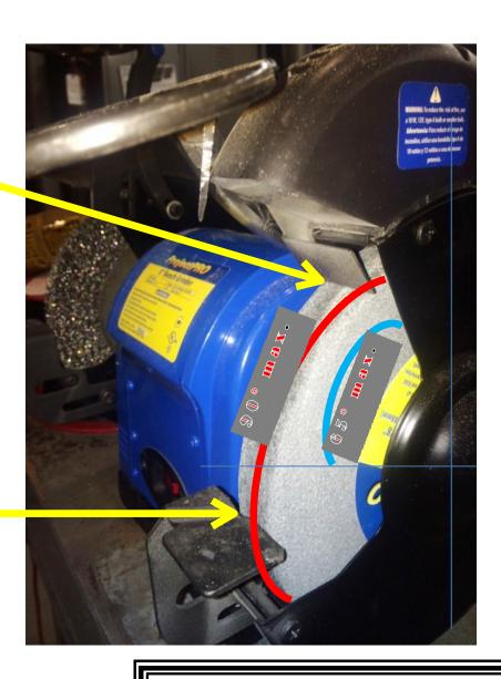
The opening of the wheel guard must not exceed 90° total, and the exposure shall begin at a point not more than 65° above the horizontal plane of the wheel spindle.
