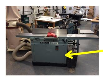
The power transmission system is located inside the cabinet.
