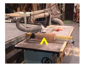
Self-adjusting blade guard must be in place and in lowered position when prior to using saw.
