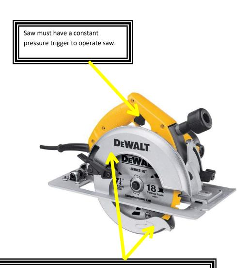
Saw must be equipped with guards both above and below the base plate. Lower guard must automatically retract when the saw is withdrawn from the workpiece.
