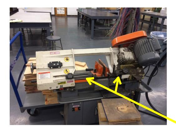
Adjust guards for saw blade so that unused portion of blade is covered.
