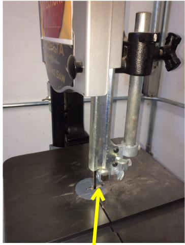
Covers need to be closed and secure before starting saw.
