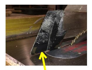
Spreader should be used when performing rip cuts. Antikickback pawls to be used to hold back wood in event saw kicks back wood.
