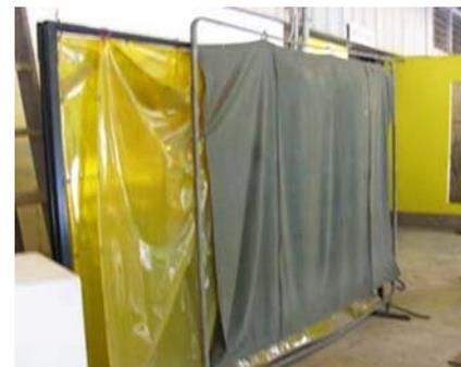
*\*Welding blankets and curtains are required to be listed, approved, or the equivalent for such use. One such approval includes ANSI/FM 4950, American National Standard for Evaluating Welding Pads, Welding Blankets and Welding Curtains for Hot Work Operations.*
