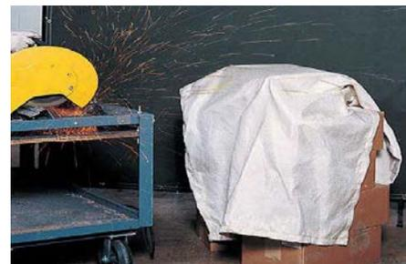
**Welding Pads:** A welding pad is heat-resistant fabric designed to be placed directly under a hot work operation such as welding or cutting. Welding pads are intended for use horizontal applications with severe exposures such as that resulting from molten substances of heavy horizontal welding.
