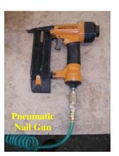
have a safety device on the muzzle to prevent the tool from ejecting fasteners, unless the muzzle is in contact with the work surface.
