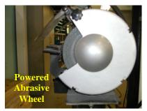
sound cracked or dead, they could fly apart in operation and so must not be used. A sound and undamaged wheel will give a clear metallic tone or "ring."
