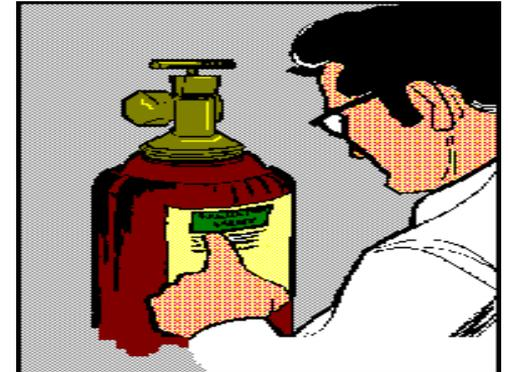
**Never rely on the color of the cylinder for identification.** Color coding is not reliable because cylinder colors may vary with the supplier. Additionally, labels on caps have little value because caps are interchangeable. The labels should be color coded to distinguish hazardous gases (such as flammable, toxic, or corrosive substances) (e.g., a yellow background and black letters).
