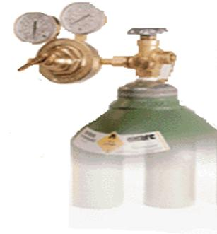
If there is any question as to the suitability of a regulator for a particular gas, check with Environmental Health and Safety Services or call your vendor for advice. After the regulator is attached, the cylinder valve should be opened just enough to indicate pressure on the regulator gauge (no more than one full turn) and all the connections checked with a soap solution for leaks. **Never use oil or grease on the regulator of a cylinder valve.**
