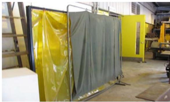
\*Welding blankets and curtains are required to be listed, approved, or the equivalent for such use. One such approval includes ANSI/FM 4950, *American National Standard for Evaluating Welding Pads, Welding Blankets and Welding Curtains for Hot Work Operations.*
