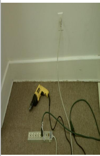
Power tool – extension cord – power strip- outlet
