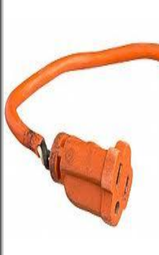
Damaged Cord at plug
